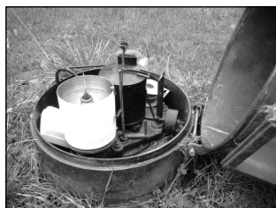
Tilting syphon rain recorder - part of the meteorologists essential equipment.
